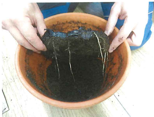
Photo No. 2 and 3 – The roots have not penetrated the Planter Eco foil
